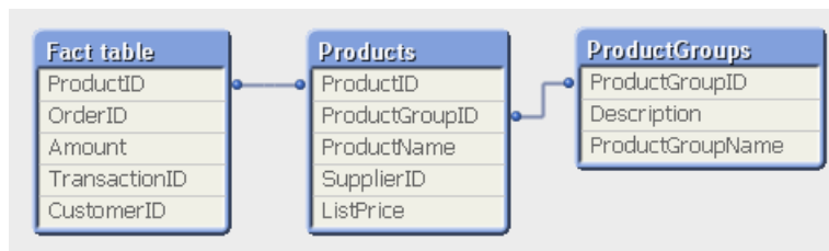
Figure 4. A product group table linked to a fact table via the product table in a standard solution.
